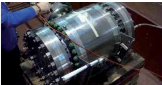
Fugitive emission testing
