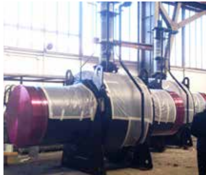
56" (1400 mm) Fully Welded valve
