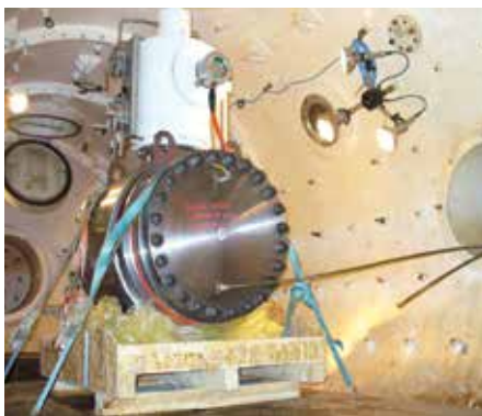
Hyperbaric testing through external subcontractor
