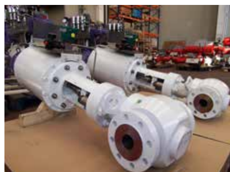
16" (400 mm) Class 600 Actuated Rising Stem Ball Valves
