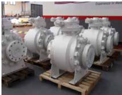
20" (500 mm) class 300 side entry valves
