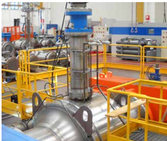
In-house testing facilities for valves up to 1600 mm (64" )
