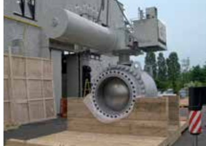
48" (1200 mm) Class 600 valve with Electrohydraulic actuator
