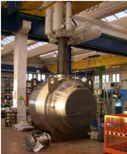
56" (1400 mm) Fully Welded, Class 600 valve
