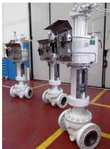
16" (400 mm) Class 900 Actuated Rising Stem Ball Valves
