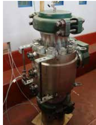
Hydraulic Shell & Seat Test on a 18" (450 mm) Class 2500 Uprated valve
