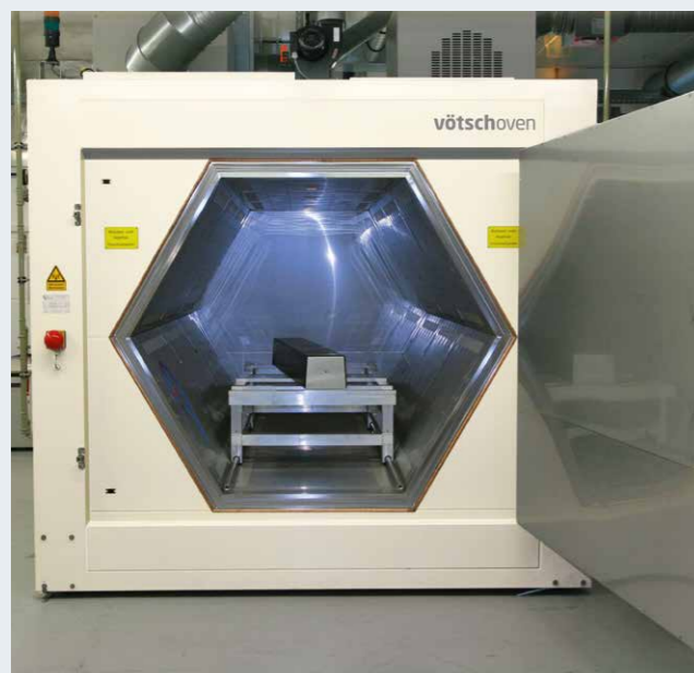
Curing System VHM 180/300 for CFRP structures in the aerospace industry
