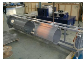
Special Dual Shaker Coupling Test Jig
