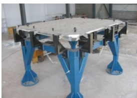
3.5 x 3m HE with 16 Ton Load Support and Guidance System
