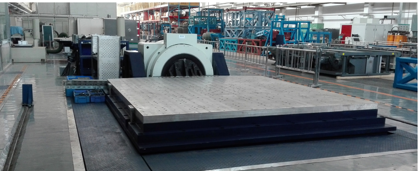
Customized slip table with 350kN vibration testing system
