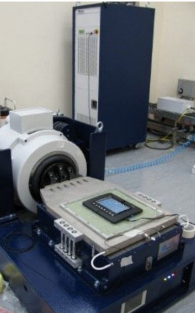
Product design reliability testing on an industrial handheld tablet by a M124M shaker with 500 x 500 mm slip table.
