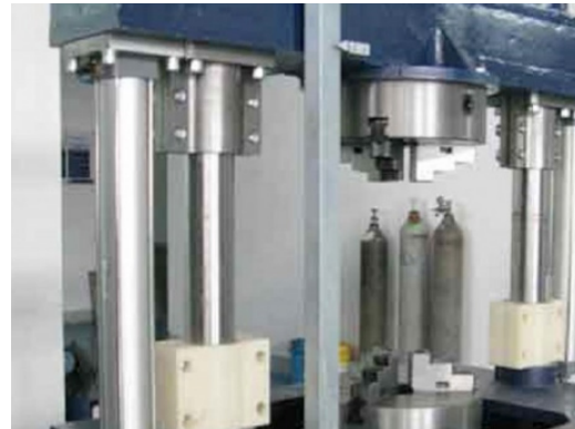
Aircraft landing gear suspension dampener fatigue test carry out on a customized LS Series shaker unit with adjustable clamping jig for different DUT length. The system is capable of achieving continuous 90mm peak to peak displacement.
