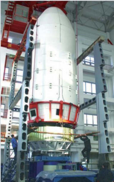
The H3580A 350kN system coupled with our customized design 2.5m head expander and slip table, capable to take up dynamic payload of up to 5 ton.
