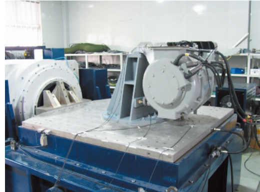
High intensity vibration testing on the 250 kgf high speed train traction motor is carried out by the H Series H1859A shaker unit to validate its system performance and conformance to its criteria under abnormal field conditions.
