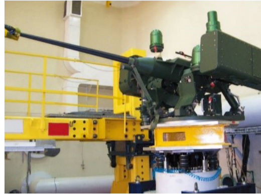
The H128A (100kN) shaker designed with a customized head expander with load support and guidance for dynamic lateral restraint to test the 2.5 ton turret payload.
