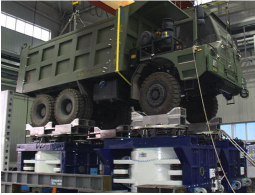
The world largest high performance 4 Poster vibration test system with four 350kN vibration test systems, successfully applied to carry out vibration test on mining vehicles.
