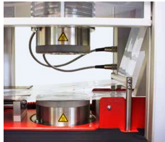
Precise film guiding to avoid any crinkles or folding of the testing film.
