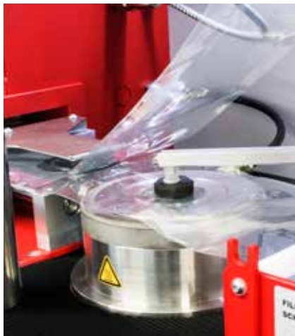
Monitored sample placement directly into the center of the die.
