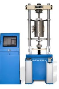
All modifications of CREEP test systems manufactured by us are designed so that the customer can fully rely on its function and accuracy with long-term constant loading (material flow) with force or stress, including elongation and at a constant homogeneous temperature in a high-temperature furnace. Intuitive and trouble-free use of test software designed for long-term tests produced by LABORTECH guarantees you a reliable declaration of results even after 100,000 hours of continuous loading.
