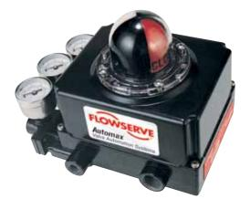
The Automax Apex 8000 positioner provides outstanding control for a wide range of valves and dampers. The twostage pneumatic relay provides fast, sensitive response characteristics to meet demanding control objectives. It may be used with 3-15 psi pneumatic control signals or fitted with an I/P transducer for 4-20 mA signals. The Apex 8000 is available with many options including position feedback limit switches, 4-20 mA position feedback transmitter and our UltraDome Visual Position Indicator.
