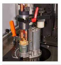
Tooling allows for flexible rotation and indexing of starter orientation. Quick clamp tooling rings optimize model changeover timing. With pneumatic clamp and available automatic solenoid contact head with radial, rotational, and height adjustment allowing for maximum versatility and productivity.
