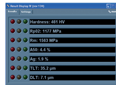
Result of a 3MA inspection
